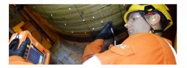
INSONO™ is ICR's advanced non-destructive inspection system. Using acoustic inspection techniques including pitch and catch, resonance, and mechanical impedance analysis, INSONO™ identifies critical issues such as delaminations within the laminate and disbonds along the bond line. Designed to meet industry demands, it ensures repair validation throughout the design life and supports life extension assessments beyond original specifications.
