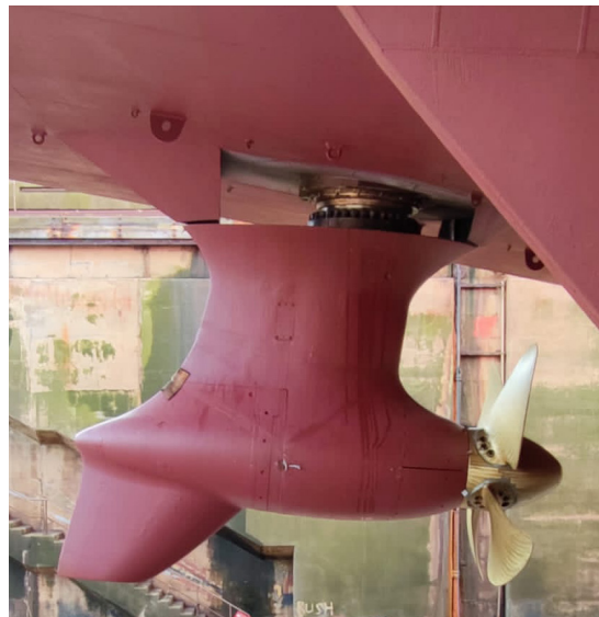
Reassembled port side thruster, post machining.
