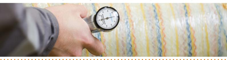
ICR's engineered composite division has over twenty-five years' experience in the provision of composite repairs. We offer bespoke, engineered repair solutions capable of rehabilitating damaged pipework, pipelines and structural components using either glass or carbon fibre stitched cloths along with a variety of two-part epoxy resins.
