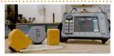
**INSONO** is a Non-Destructive Testing technique for inspection of composite repairs applied to metallic components, validated by the welding Institute (TWI) with patent and UKAS accreditation pending. It has been developed to validate the condition and integrity of composite repairs providing operators with assurance in the installation, long-term performance, and evidence to support life extension of the repair.
